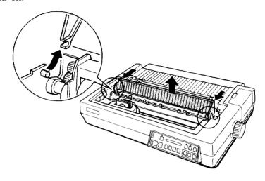
4. Hold the pull tractor with the gears to the right. Fit the rear notches on the tractor over the rear mounting rods on the printer, as shown in the following illustration.
